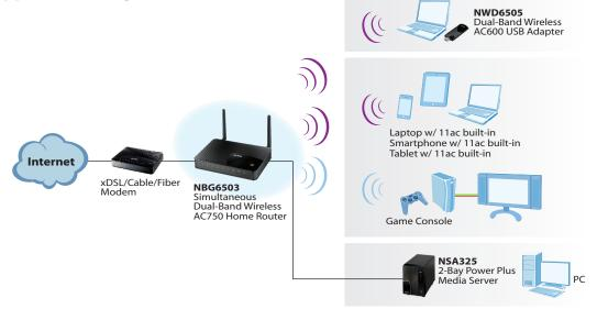
5 GHz 2.4 GHz Ethernet HDMI/RCA Cable
