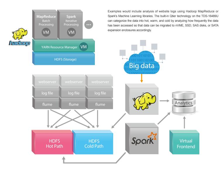
Use Spark Streaming to perform predictive analytics by analyzing a website's workloads, click rates, and data from Global CDN. Dynamically adjusting system resources enables the highest system utilization to be achieved among multiple TDS-16489U units on the local network or across different deployment sites.
